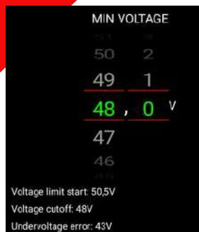
**8-Min Voltage:** Minimal and maximal voltages are set automatically, according to the battery type you choose from the menu above. You can also customize the voltage values for each Battery Type, but we recommend you use the controller within the limits of preset values.
