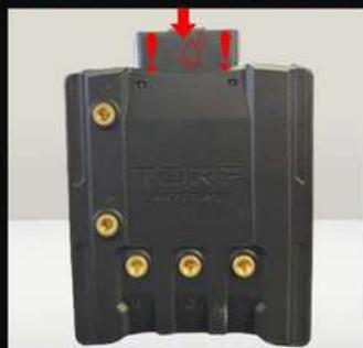
**WARNING: Water in the main connector! Turn off the bike immediately, disconnect the main connector and dry it out!**
