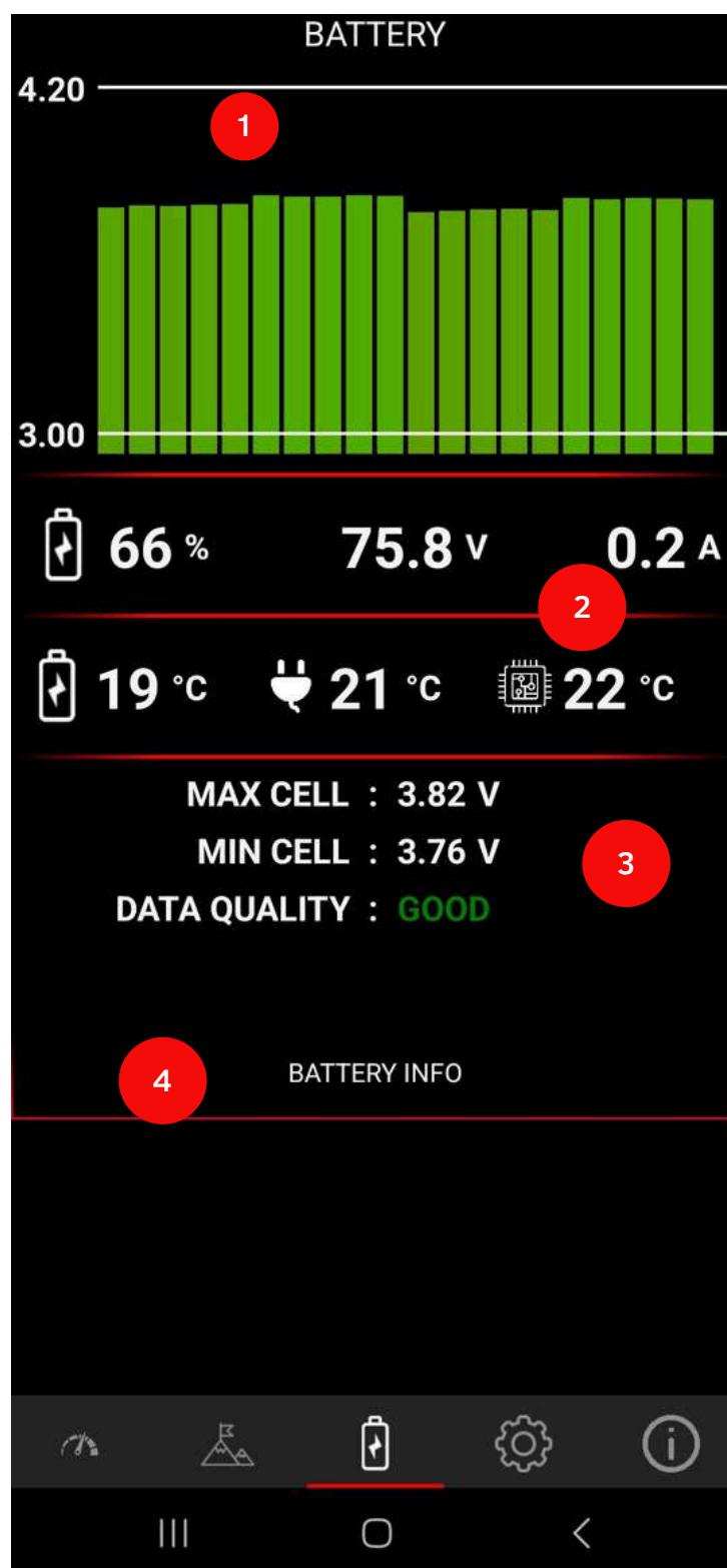
**1 - Battery Cell Voltage:** Check the voltage of each battery cell. The more the columns are aligned, the healthier the battery.
