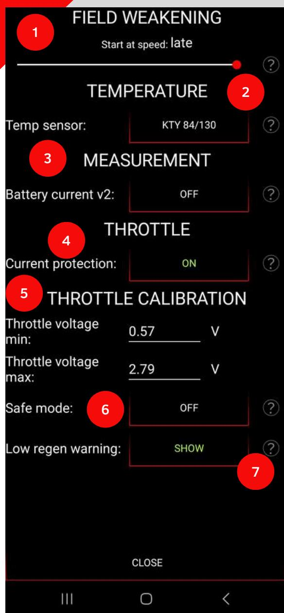
**1-Field weakening:** Set at which speed the FW is activated. It impacts motor efficiency and FW performance. For max efficiency set it to “late”.
