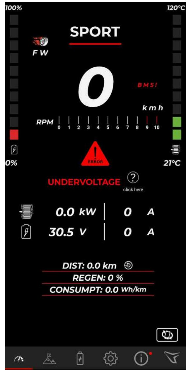
**IMPORTANT:** After the installation make sure to calibrate the throttle and motor! Go to the 5th screen of the Torp App and click the CALIBRATION button. Then follow the setup Wizard. CALIBRATION must be repeated after each firmware update!
