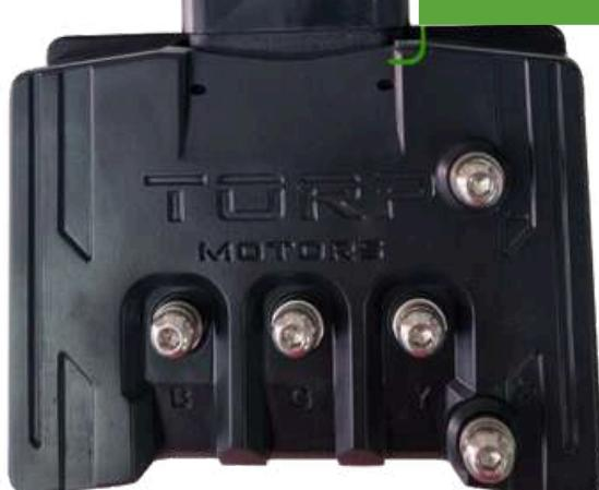
If you ever need to unplug the main connector in the future (and dielectric grease was previously applied) first clean off the old grease with alcohol contact cleaner and once dry, reapply the dielectric grease.
