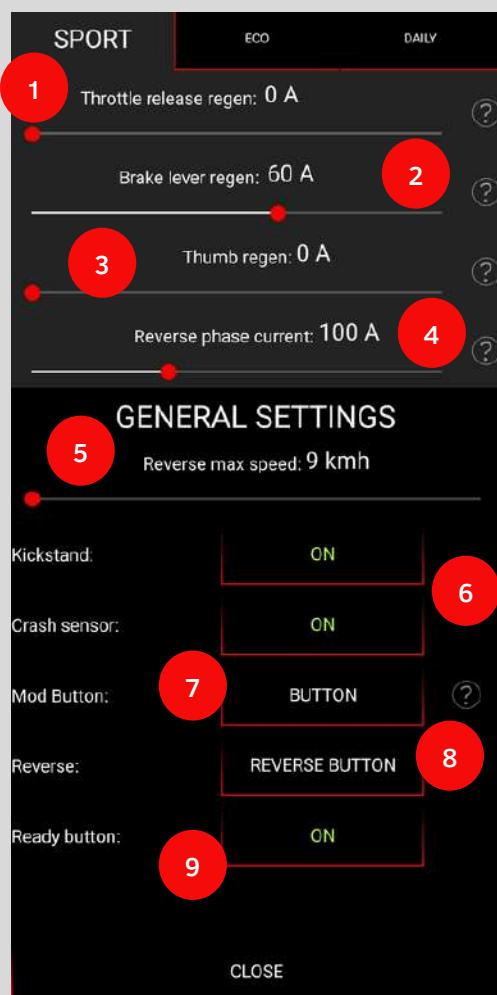
**1-Throttle release regen:** It defines the strength of the regenerative braking that is activated when the throttle is released. With this setting a small dead zone is applied to the throttle.
