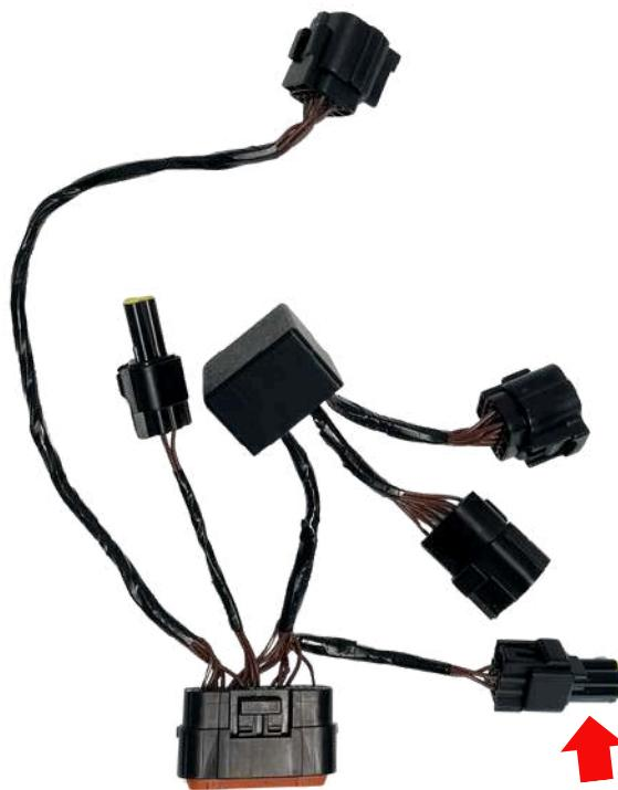
The Torp Display is being installed directly to the controller's wiring harness, as shown on the photo.
