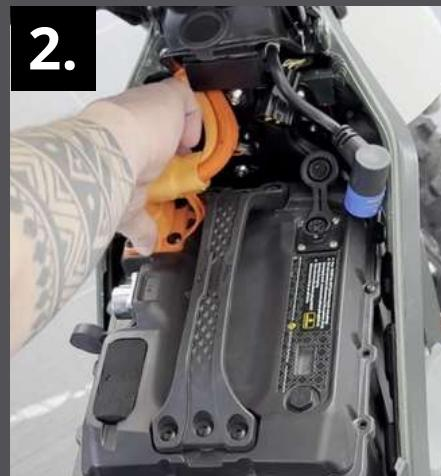
Now you can start removing the stock SurRon controller and lower the skid-plate that covers the wiring.
